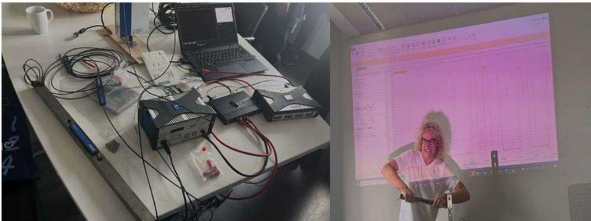
LEFT - MEASUREMENT SET-UP OF A STRAIN GAUGE, WHICH INCLUDES LOAD CELL, DATA ACQUISITION UNITS, AND COMPUTER. RIGHT - THE REAL-TIME ANALYSIS OF THE STRAIN
