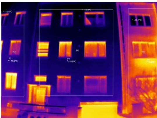
THERMAL IMAGES WERE USED TO ENRICH THE POINT CLOUD DATA
