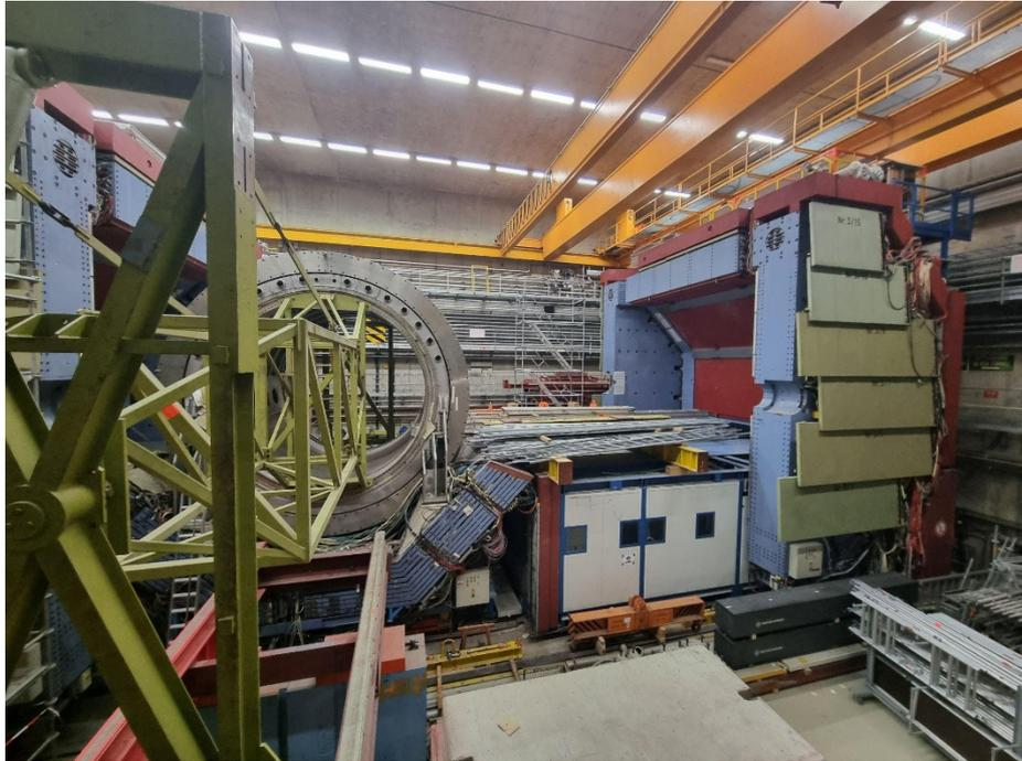
This powerful system operates deep beneath the surface, with precision being a top priority in the alignment and operation of its components. We learned about an innovative technique used to cool down the pipelines and older electromagnets, allowing the magnets to reach their full potential and extend their lifespan.
